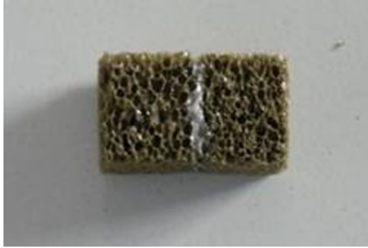
Fig. 3 Foamglas ® specimen joined by glass G7 (half-sample size 30 by 30 by 30 mm)
